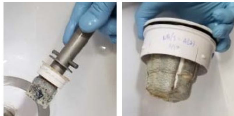
Figure 4 - Sumpless Cartridge Style with Silicon Check Valve (1 Month Operation)
